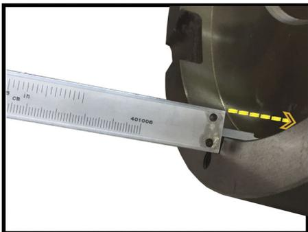
To measure the depth of your flywheel hole, start with the edge on top until you reach the clutch disc at the bottom.
